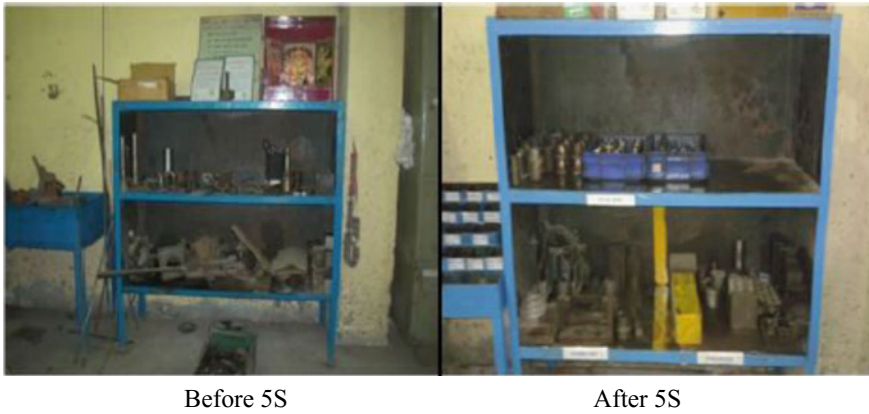
Fig. 5 Tools were placed haphazardly but after 5S everything was placed in proper way with name slip [12]
