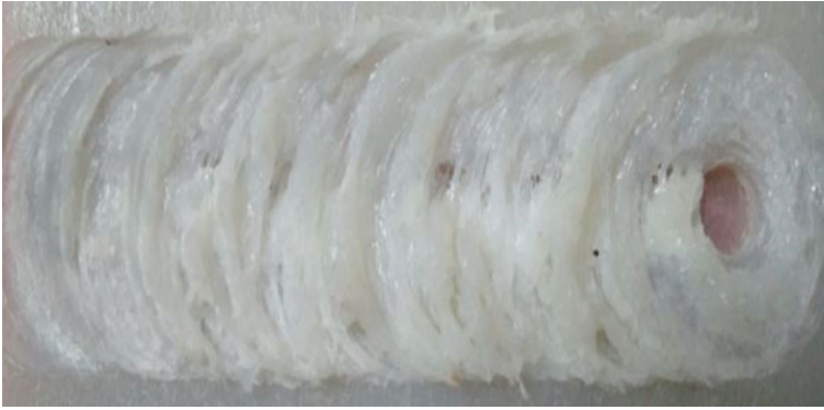
Fig. 5 Typical macrograph of weld crown at tool traverse speed of 0.6 mm/s, tool rotational speed of 600 rpm, and tilt angle of 2^\circ
