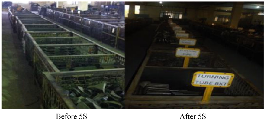
Fig. 4 Subassembly components are without nameplate, but after 5S naming was done [12]
