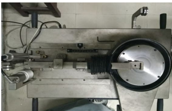
Fig. 2 Wear testing set-up (pin-on-disc)
