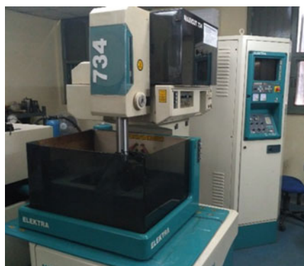
Fig. 1 Wire electric discharge machining with tool and workpiece
