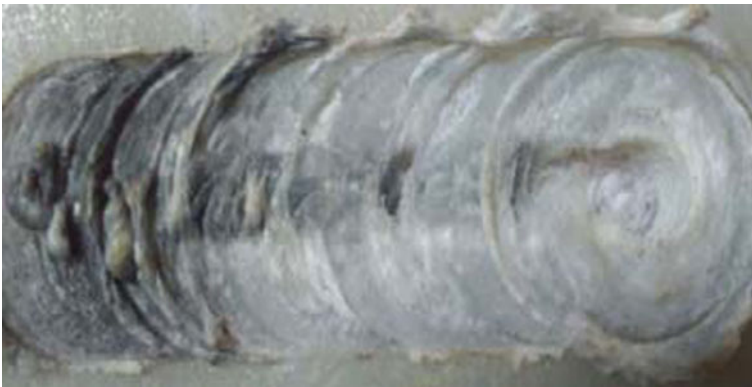
Fig. 6 Typical macrograph of weld crown at tool rotational speed of 1000 rpm, tool traverse speed 0.2 mm/s, and tilt angle of 2^\circ
