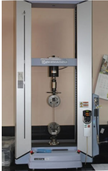
Fig. 1 Tensile testing according to ASTM D3039
