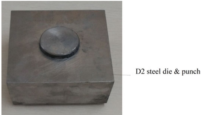
Fig. 2 D2 die steel punch and die for compacting the powders
